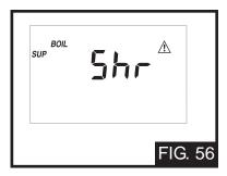
The control is no longer able to read the boiler supply sensor due to a short circuit (FIG. 56). The control will not operate the boiler(s) until the sensor is repaired. Locate and repair the problem as described in INS7141. To clear the error message from the control after the sensor has been repaired, press either the Menu or Item button.
